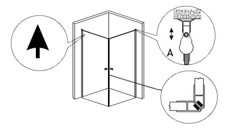
3. As Figure, drill diameter 3.2mm hole in the 200mm upper and lower ends of the aluminum profile. Screw the fixed and the adjustable aluminum by ST4\*20 screw. Cover screws with the decorative covers
