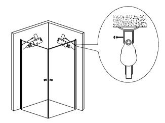
4. Installed waterproof tape under the door ,install the handle. Inject both sides of the shower cabin by Neutral silicone sealant
